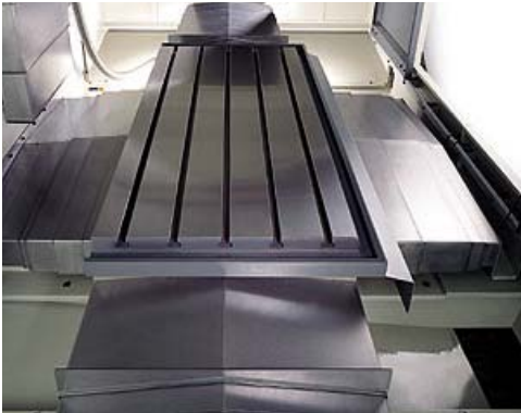
The EC-500T is a 3 axis HMC with 5 T slot table (1200 mm x 600 mm)
