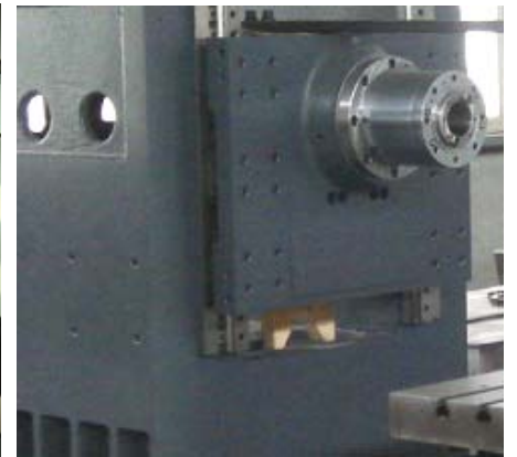
#40 inline direct-drive spindle, #50 as an option
