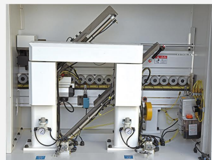
Two motors traveling on linear guides for end-trimming
