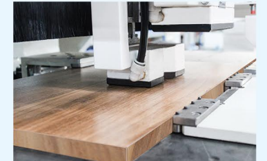
Panel hold-down device with rubber feet guarantees accurate processing
