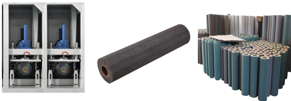
拉丝辊 (用于r工位) Roller brush (for r station)
