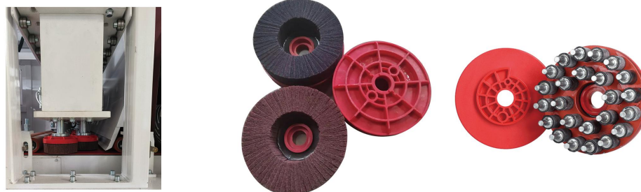
清渣锤/砂块 (用于H工位) Slag cleaning hammer / sand block (for H station)
