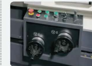
Manual operation box
