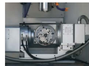
4th and 5th axis auxiliary device interface Users who wish to set up a rotary axis on the table to increase application flexibility are encouraged to contact sales representatives.
